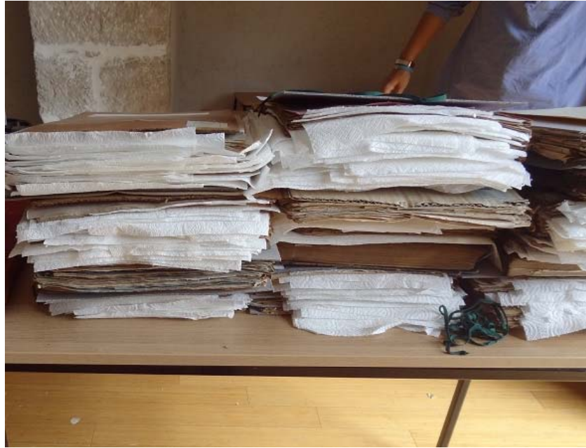
Figure 3: Moisture absorption of flooded archives materials
